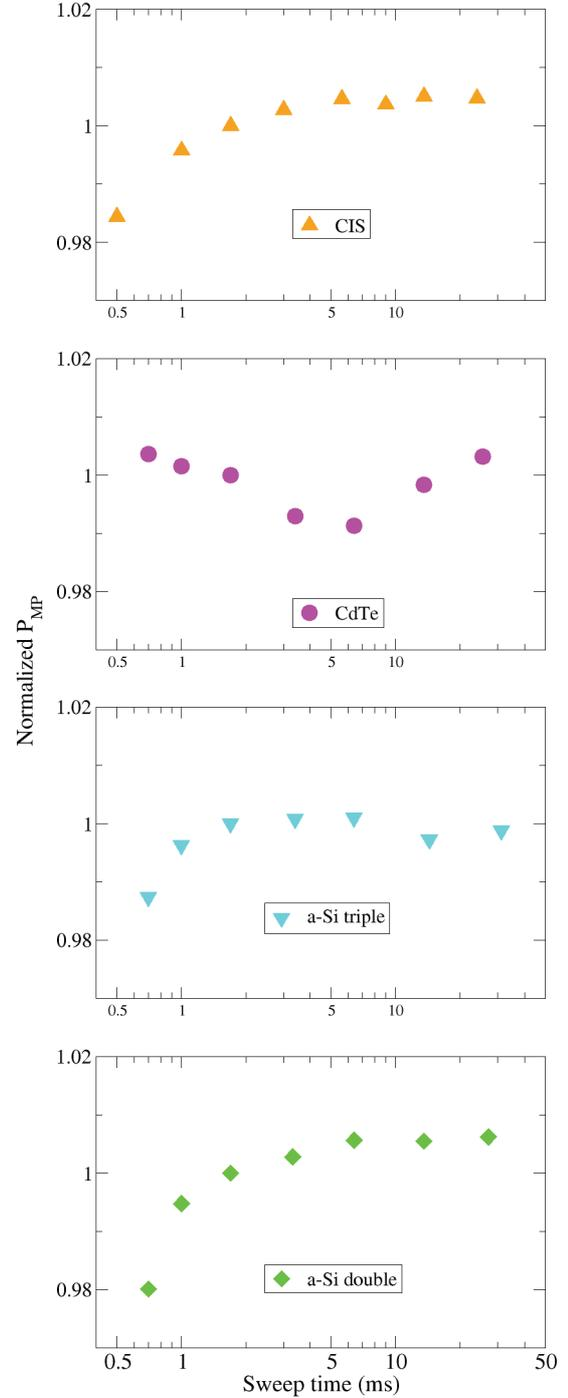
**Figure 1. The normalized maximum power of four modules with different sweep times outdoors.**
