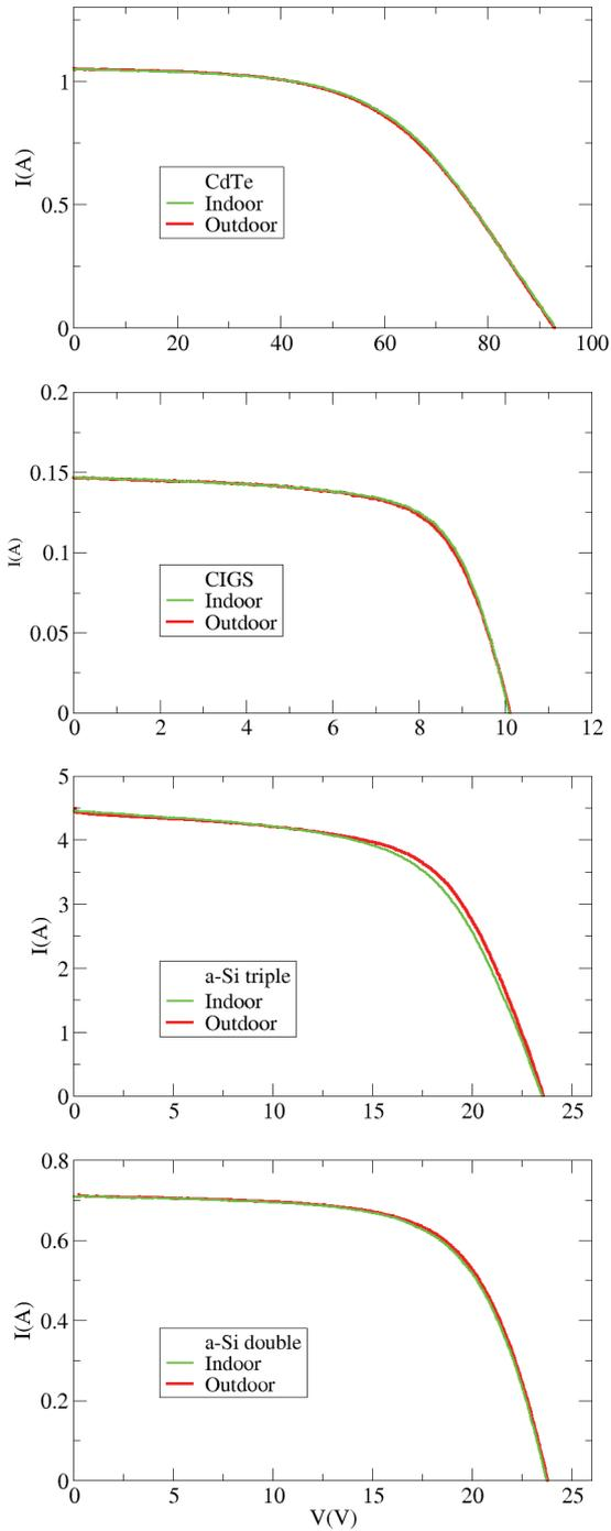
**Figure 2. The I-V curves of four modules measured indoors and outdoors.**
